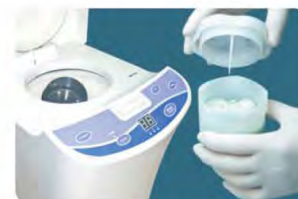
3. Close tightly the cap of mixing bowl
