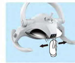
Moving near sensor points will be on or off light, the light during light on position. sensor range is 20mm-80mm
