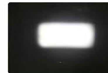
The color and color temperature for the whole light spot are the same,greatly reduce the color separation through the lens,as well as the effect to the light sensitive material.
